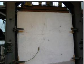
After one hour and ten minutes some cracks have appeared, and smoke started to leak through the wall. Nonetheless, this side of the wall is still safe, the wall keeps the flames at bay.
