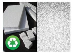
On the construction site, there is no waste from the frame structure, since the pieces are transported based on the production plans and they are all used up in the assembly of the frame structure. In the case of polystyrene concrete, some waste may be generated, but that is immediately used up together with the bulk polystyrene when pouring the slab, as illustrated in the pictures below.
