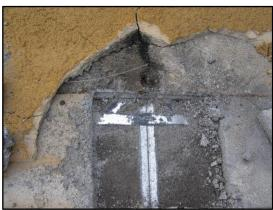
The two-hour long slab burning is depicted with only a few pictures. The 39 cm thick slab also complies with the fire safety regulations. In the case of the slab, there was no fire-proof plaster applied, the temperature reached 1000°C in this case as well.
