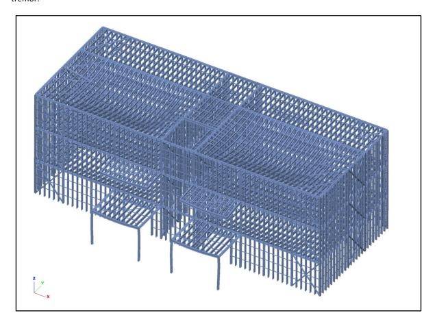
We can conclude that buildings built with Löglen walls and slabs up to low heights (2 floors), under Hungarian conditions ( $p_s = 1.00 \text{ kN/m}^2$ ,  $v_{b0} = 23.6 \text{ m/s}$ ,  $a_{gr} = 0.12*g$ ) can stand potential impacts without a separate reinforcing steel frame. In case of more floors, the application of a separate steel frame can provide the proper load capacity.
