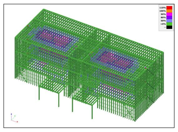
Now, let us examine the impacts on the main structural frame. It can be seen that in this case the pieces of the main structural frame serve as reinforcement and columns for corner and 'T'-shaped wall connections, providing stability for the building against different impacts, like earthquakes.
