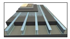
In case of a load-bearing slab, 8 cm thick polystyrene panels are fixed on the bottom of 20 cm wide steel profiles. On top of the panels, a 20 cm thick bulk polystyrene concrete layer is poured. On top of all these, first a weight-distribution grid is placed then a 4 cm thick polystyrene concrete layer and a 5 cm thick estrich concrete layer is poured. The floor cover is placed afterwards.
