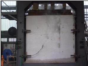
Near the end of the experiment, at 1046°C, we can see that in the middle picture below, on the right side of the wall, there is a strong leakage of smoke, while the left side is still left visibly undamaged. Also, we can observe (rightmost picture) that the wall has bulged due to the long lasting pressure.
